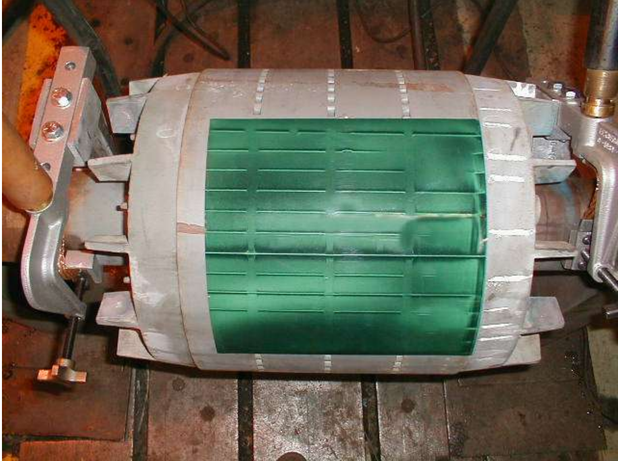
A sample image of the Magnetic Paper used with a Lexseco Core Loss Tester to identify faulty bars on a Squirrel Cage Rotor
